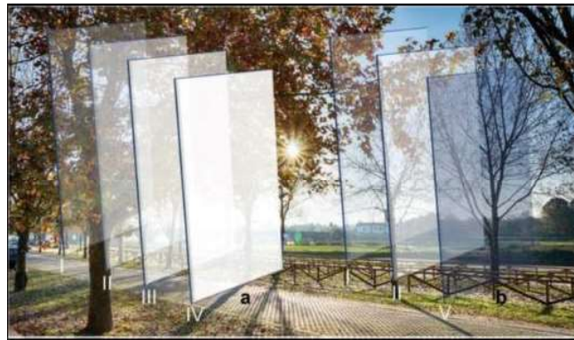
Figure 6: a) Electrochromic system, which changes its transparency, becoming semi-transparent; b) Thermochromic system, which adjusts its colour and opacity in response to sunlight. Source: Lima et al., 2025.
